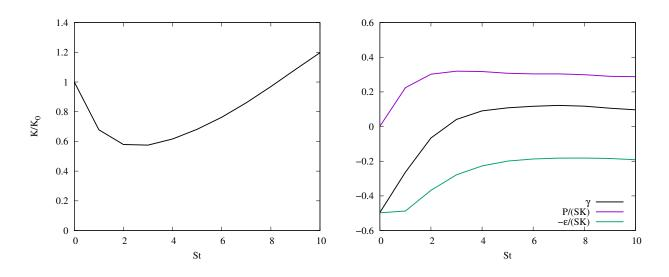
Figure 1. Evolution of the normalized turbulent kinetic energy  $K/K_0$  with normalized time St (left) as well as the growth rate of the turbulent kinetic energy  $\gamma$ , the normalized production rate P/(SK), and the normalized dissipation rate  $\varepsilon/(SK)$  (right).
