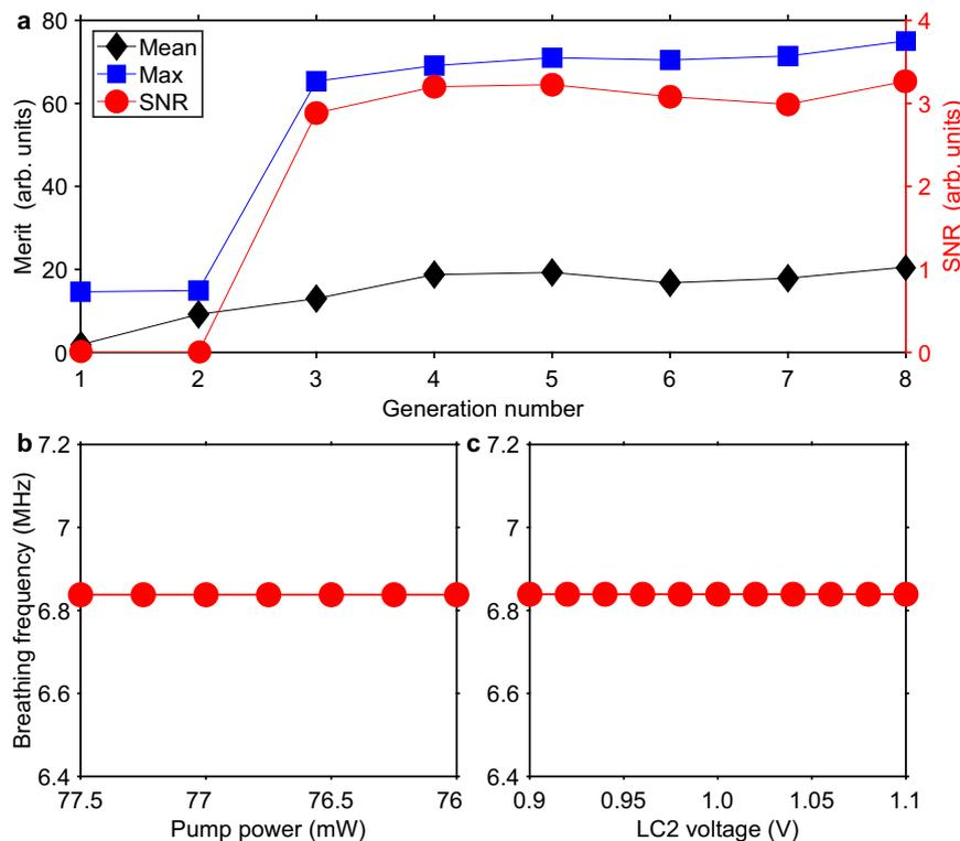
**Fig. 4 | The machine-learning results.** **a** Evolution of the mean (black diamonds) and best (blue squares) merit scores of the individuals for each generation. Also shown is the corresponding evolution of the SNR (signal-to-noise ratio) of the
