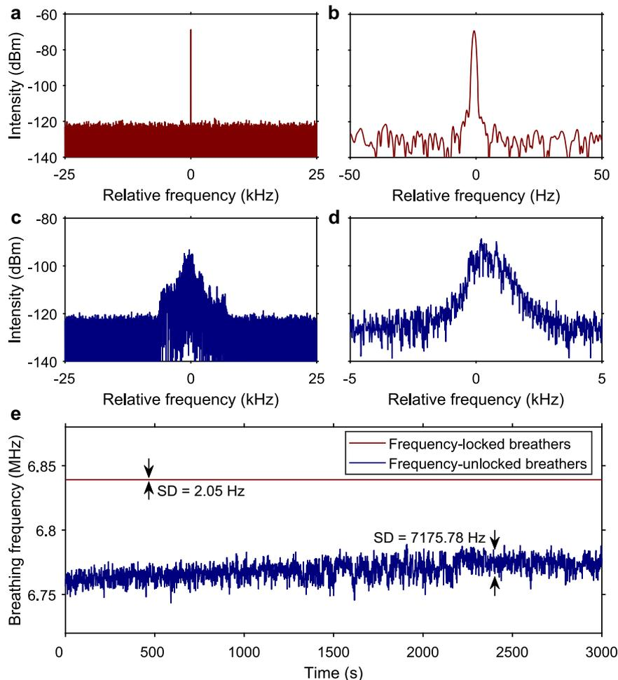
**Fig. 3 | RF spectral measurements of the breather states shown in Fig. 2.** The reference frequency is one-fifth of the fundamental repetition frequency. **a, b** Single-mode oscillation of the breathing frequency when frequency locking occurs measured over spans of 50 kHz and 100 Hz, respectively. **c, d** Unstable multimode oscillation of the breathing frequency measured
