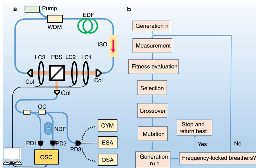
**Fig. 1 | The experimental configuration.** **a** The breather fibre laser setup. WDM wavelength-division multiplexer, EDF erbium-doped fibre, ISO isolator, LC liquid crystal phase retarder, PBS polarisation beam splitter, Col collimator, OC optical coupler, NDF normally dispersive single-mode fibre involved in the dispersive
