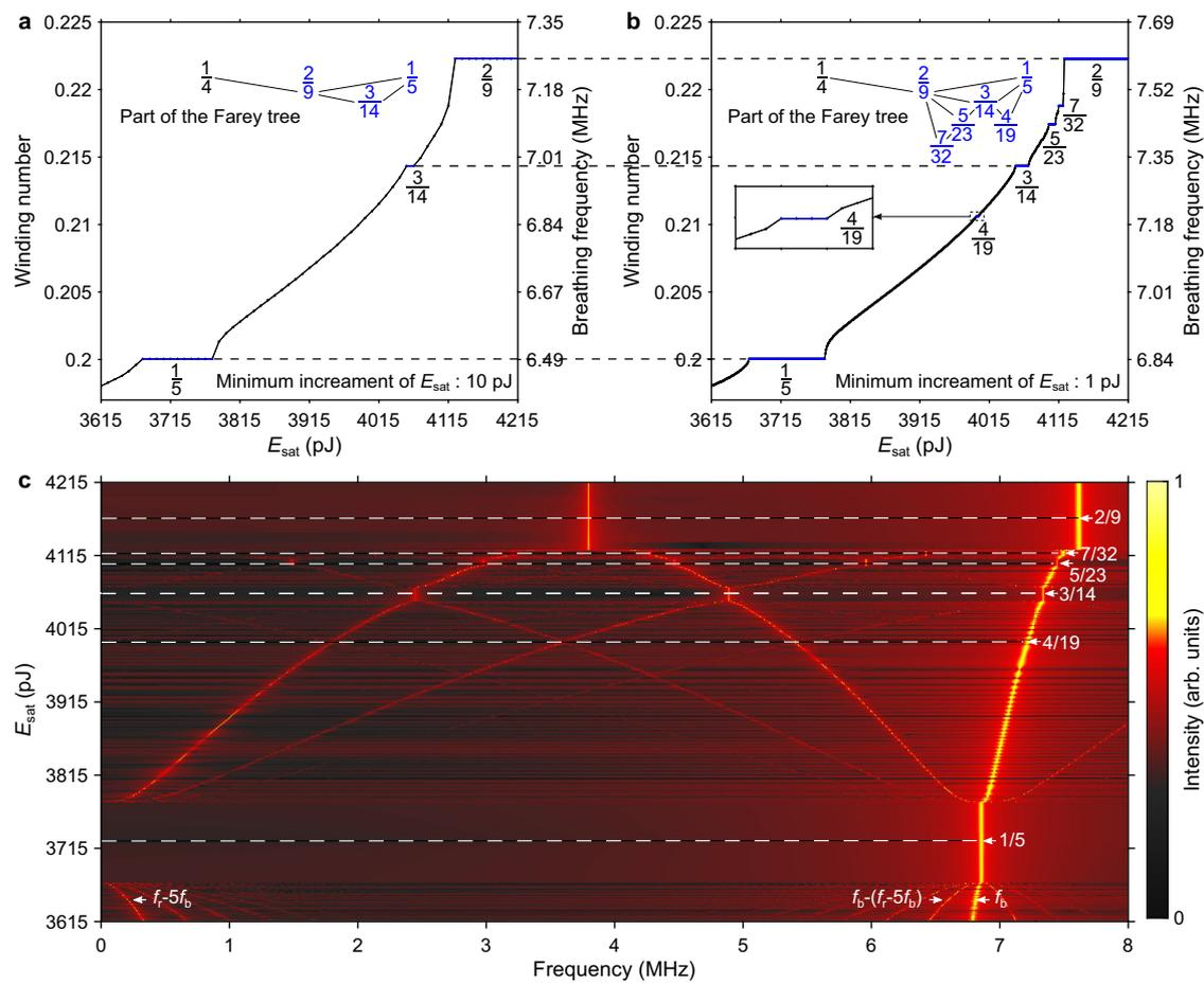
**Fig. 6 | Farey tree and devil's staircase observed in the numerical simulations.** **a, b** Breathing frequency (winding number) as a function of the gain saturation energy  $E_{\text{sat}}$  (related to the pump power in the experiment) varied with a step of 10 and 1 pJ, respectively. With the smaller step, more plateaux are observed, evidencing a fractal pattern. In the insets are shown the parts of the Farey tree containing
