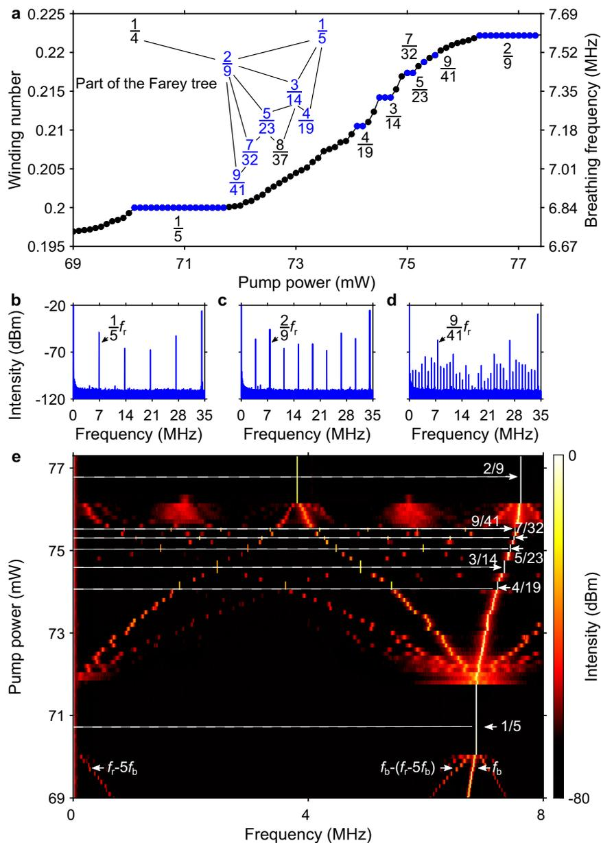
**Fig. 5 | Farey tree and devil's staircase measured in experiments.** **a** Measured breathing frequency (winding number) as a function of the pump power. In the inset is shown the part of the Farey tree containing the observed winding numbers (blue). **b–d** RF spectra measured with the ESA showing dense frequency combs for the frequency-locked states corresponding to the winding numbers  $1/5$ ,  $2/9$  and  $9/$
