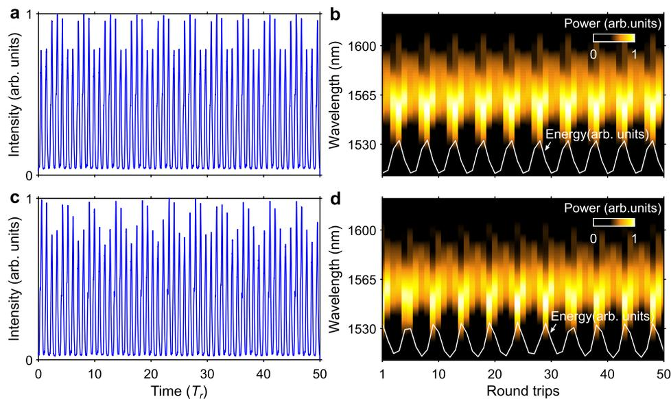
**Fig. 2 | Two different breather operations of the laser observed over 50 cavity roundtrips. a, b** Frequency-locked breather state showing a well-defined periodicity, and **c, d** frequency-unlocked breather state featuring degraded periodicity. Panels
