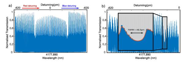
Fig. 3. (a) Wavelength scan (ramp up and ramp down) of the ring resonance with a cw QCL. The ring resonance at one specific wavelength can be clearly distinguished from the Fabry-Perot resonances, which occur due to the waveguide facet at input and output coupling. (b) Zoom-in on the ring resonance.
