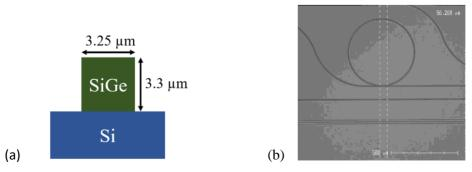
Fig. 1. (a) SiGe platform used for the ring resonator. (b) SEM picture of the ring resonator.
