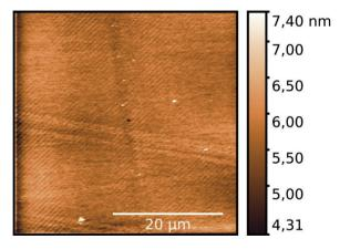
**Fig. 2.** An AFM image of the surface topography of sample SN492. The regular fluctuations are attributed to instrumental effects for a very flat surface. (For interpretation of the references to colour in this figure legend, the reader is referred to the web version of this article.)
