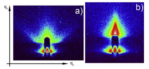
**Fig. 12.** 2D GISAXS pattern recorded at an incident angle 0.05° from: a) unirradiated sample SN490, b) irradiated sample SN490\*. Red colour — high intensity, blue colour — low intensity. (For the colour version of this figure, the reader is referred to the web version of this article.)
