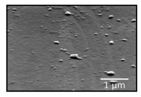
**Fig. 3.** A secondary electron SEM image of the surface topography of sample SN490 showing presence of contaminants.
