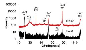
**Fig. 10.** XRD results for sample SN489 (bottom): unirradiated UO $_2$  film on LSAT (111) substrate analysed on a D8 Bruker diffractometer and sample SN489\* (top): irradiated UO $_2$  film on LSAT (111) substrate analysed on a Rigaku D/MAX 2500 diffractometer. The peaks at ~33 and 47° can correspond to 200 and 220 reflections from the UO $_2$  film or 220 and 400 reflections from the LSAT substrate.
