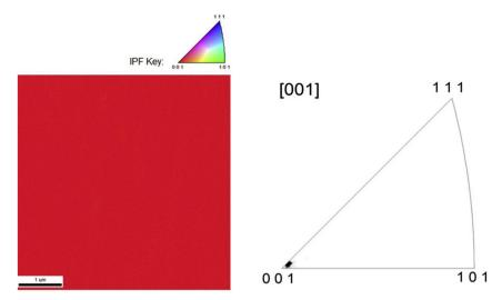
Fig. 11. EBSD results for sample SN491: the inverse pole figure map (left) and the corresponding inverse pole figure triangular diagram [19] (right). (For interpretation of the references to colour in this figure legend, the reader is referred to the web version of this article.)
