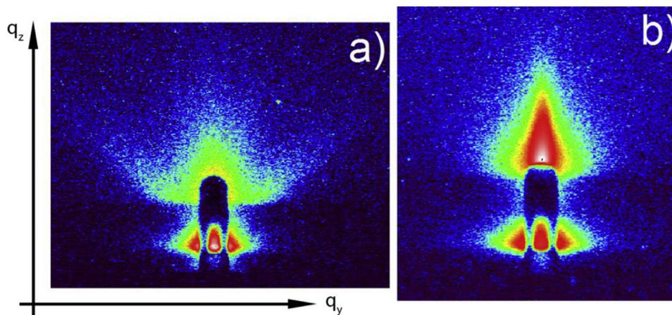
**Fig. 12.** 2D GISAXS pattern recorded at an incident angle  $0.05^\circ$  from: a) unirradiated sample SN490, b) irradiated sample SN490\*. Red colour – high intensity, blue colour – low intensity. (For the colour version of this figure, the reader is referred to the web version of this article.)
