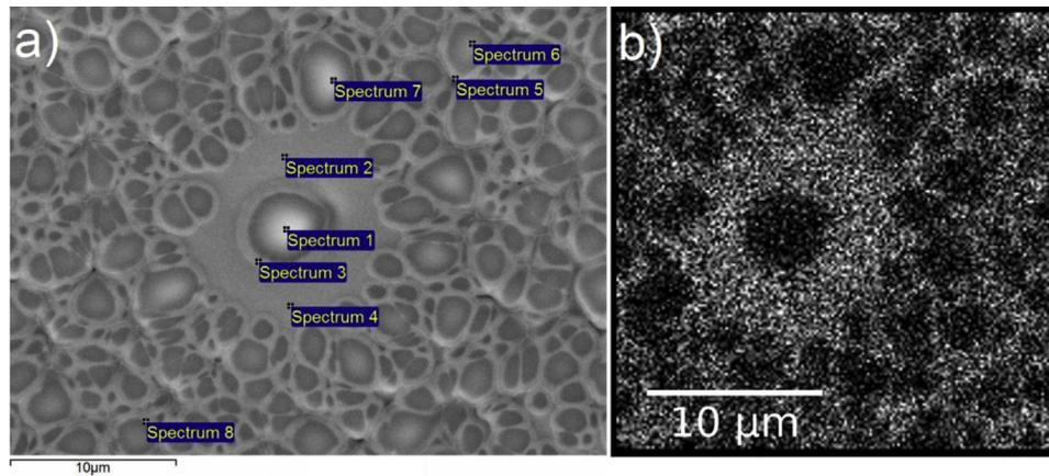
**Fig. 9.** a) A secondary electron SEM image showing the EDX elemental analysis points, with the quantification results shown in Table 3, and b) EDX map of the U  $M\alpha_1$ -line signal on the surface of irradiated sample SN492\*.
