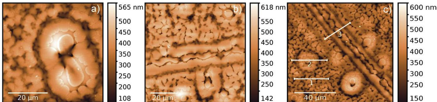
Fig. 7. AFM images of irradiated samples: a) SN489\*, b) SN490\*, c) SN492\*. (For interpretation of the references to colour in this figure legend, the reader is referred to the web version of this article.)
