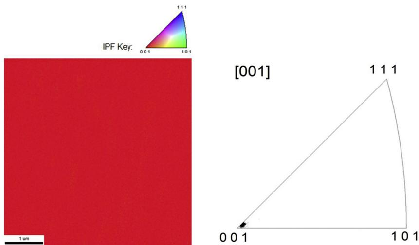
**Fig. 11.** EBSD results for sample SN491: the inverse pole figure map (left) and the corresponding inverse pole figure triangular diagram [19] (right). (For interpretation of the references to colour in this figure legend, the reader is referred to the web version of this article.)
