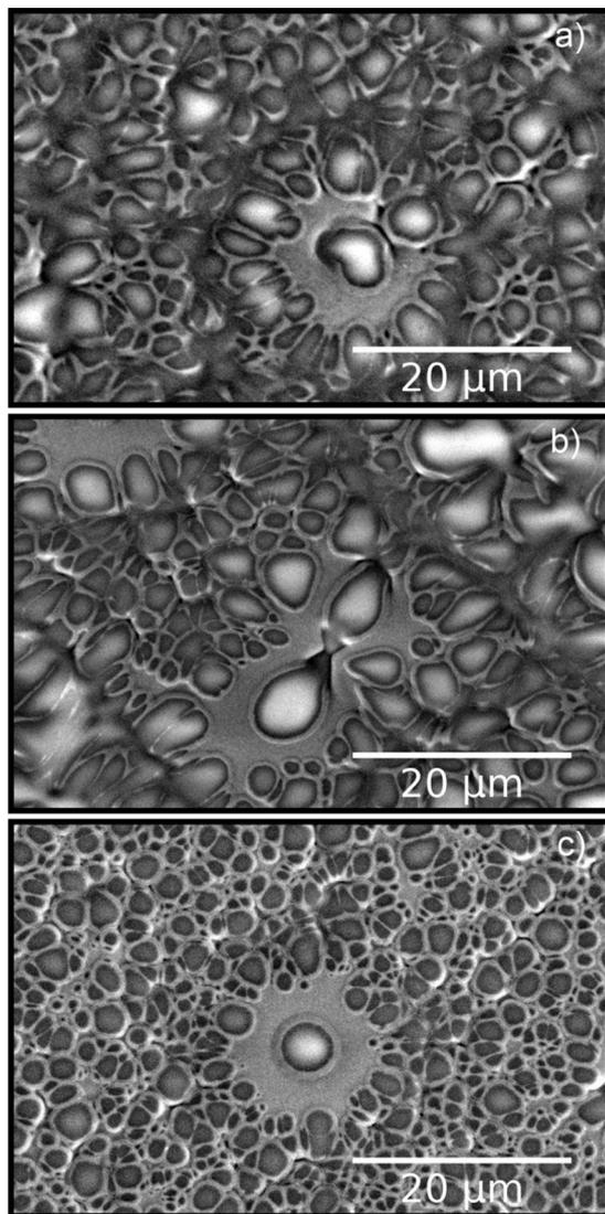
**Fig. 5.** Secondary electron SEM images of irradiated samples: a) SN489\* (preferentially (210) UO<sub>2</sub>, originally), b) SN491\* (UO<sub>2</sub> in (001), originally), c) SN492\* (mostly (111) UO<sub>2</sub>, originally).
