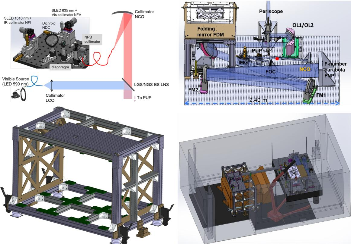
Figure 1: **Top-Left:** CAD model of the testbench NGS light source and a sketch of the LGS light source. **Top-Right:** GPAO test bench telescope simulator CAD view, with the Corrective Optics support structure on the top-left. Optical elements have all a 3-letter acronym recalling their functions (see text for details). **Bottom-Left:** WFS support structure CAD view. **Bottom-Right:** The GPAO testbench in its clean room.
