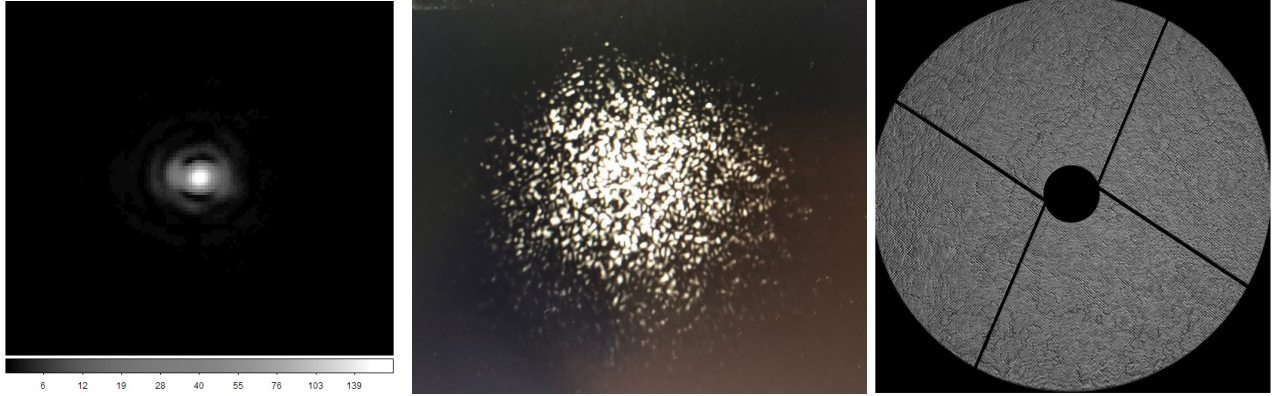
Figure 4: Left: GPAO testbench PSF core (hyperbolic arc-sinus scale), measured with the visible bench camera. Middle: visible PSF with the phase mask in place (screen shot). Right: Pupil visualization, showing the UT mask (in black) in front of the phase mask (giving an uniform grainy pattern).
