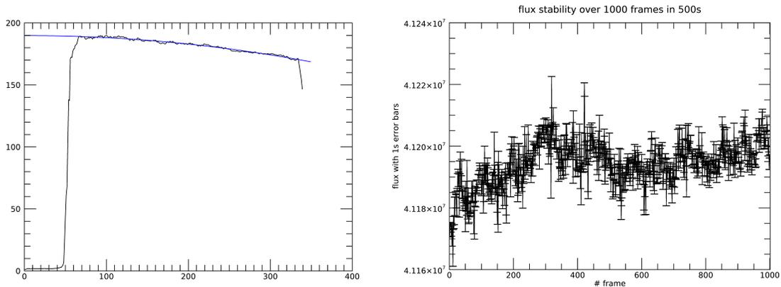
Figure 5: **Left:** Pupil illumination homogeneity, showing an azimuthally-integrated pupil flux (in black, arbitrary units) compared to a polynomial fit (blue curve) as a function of detector pixel number. **Right:** Flux averaged over the full pupil as a function of time.
