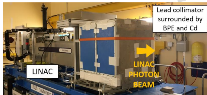
90 91 Figure 1: Saturne LINAC with collimator and neutron shielding.
