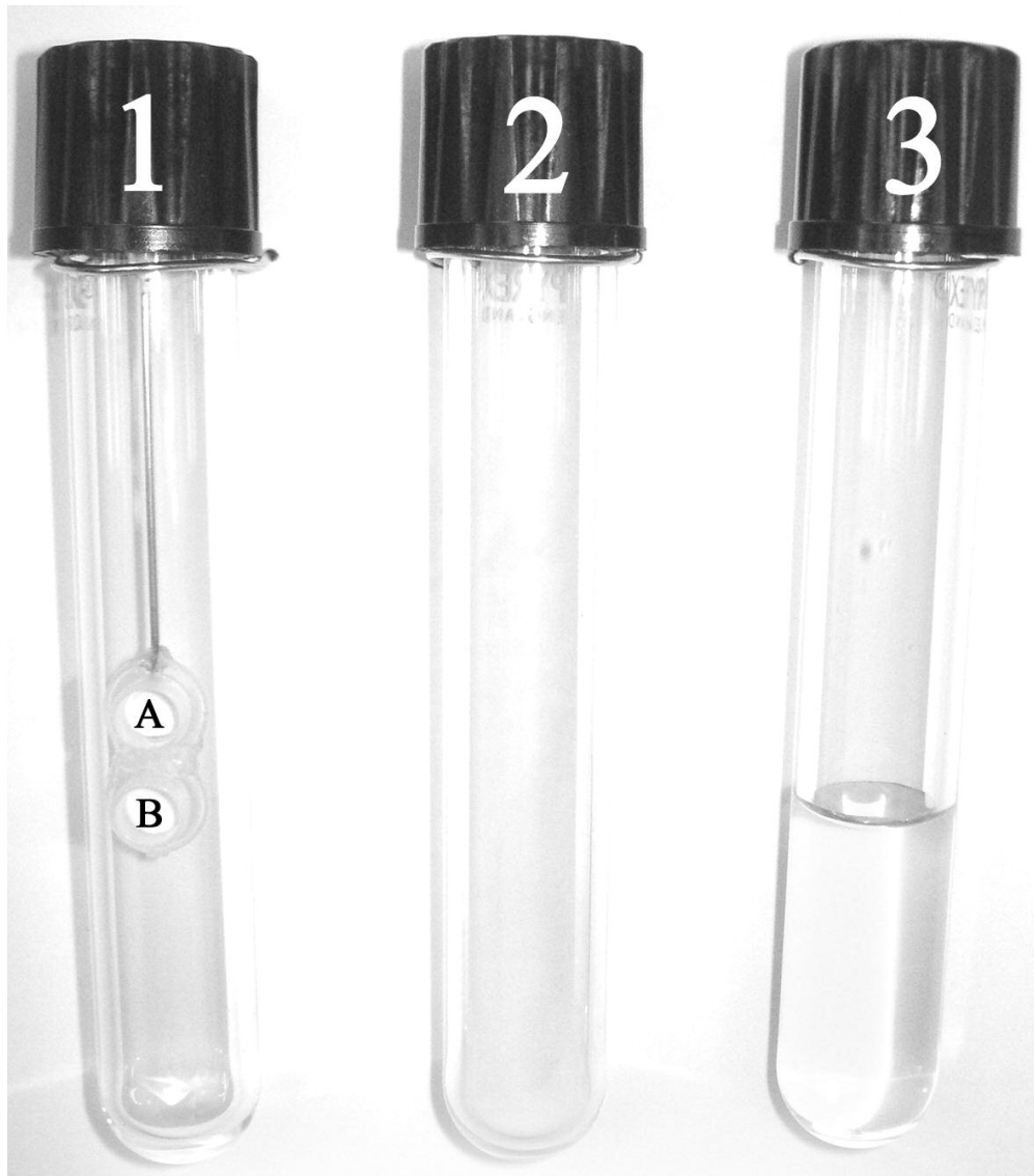
Figure 2 : Sposensor detection kit. Tube one is the Starter/Controller that contains control and sensing spores (disk A and B respectively), each immobilized on a Watman 3 paper discs placed in plastic rings. Tube two is the Developer, it contains dehydrated growth medium which is re, hydrated with 2 ml of the water solution to analyse. In such condition germination and detection are performed in one step. Tube three is the Killer which contains 2ml of bactericidal solution composed of \text{CuSO}_4 (108mM), ascorbic acid (180mM) and NaCl (1M).
