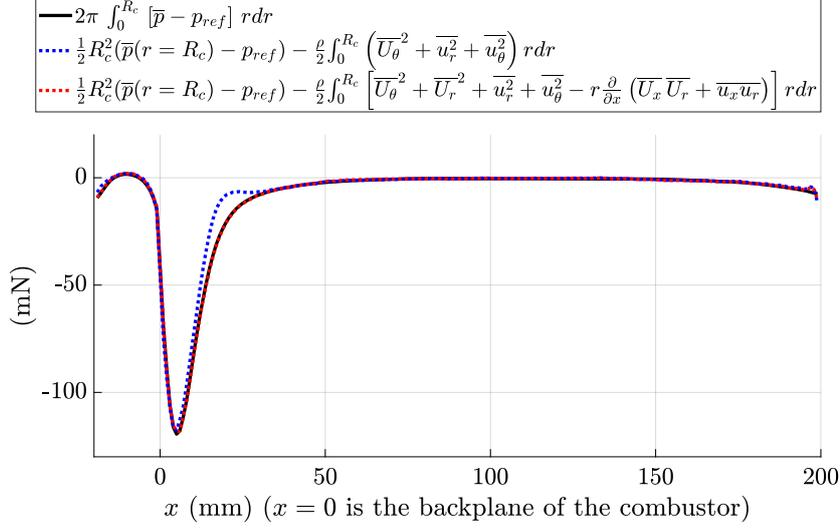
Figure 12: Axial evolution of different pressure correction expressions. Blue, Eq. (35); red, Eq. (56). The reference line is in black.  $p_{ref} = 101\,325.3$  Pa in the chamber ( $x > 0$ ) and  $p_{ref} = 101\,405$  Pa inside the injector ( $x < 0$ ).
