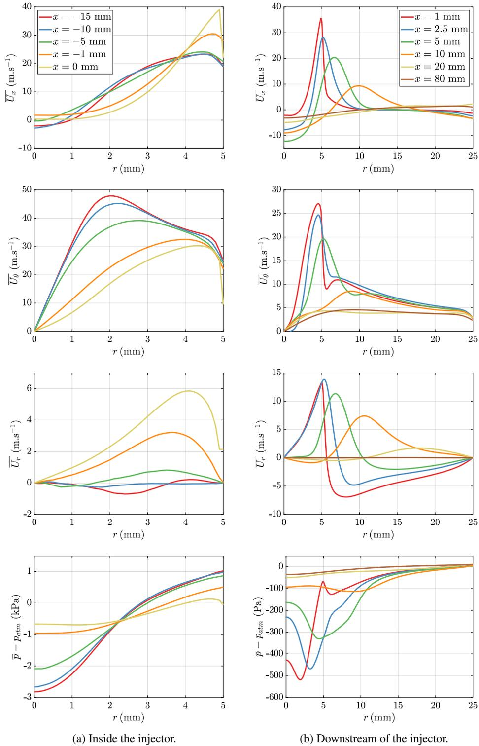
Figure 9: Radial profiles of the mean axial velocity  $\bar{U}_x$ , tangential velocity  $\bar{U}_\theta$ , radial velocity  $\bar{U}_r$  and pressure  $\bar{p} - p_{atm}$ . The four plots on the left show these variables for five axial locations inside the injector, the four plots on the right for six axial sections in the chamber.
