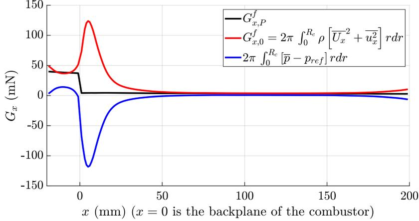
Figure 11: Evolution of  $G_{x,P}^f$  and its constituents (Eq. (53)) in the axial direction. The sudden expansion corresponds to  $x = 0$ . The reference pressures are set to  $p_{ref} = 101\,325.3$  Pa in the chamber ( $x > 0$ ) and  $p_{ref} = 101\,405$  Pa inside the injector ( $x < 0$ ).
