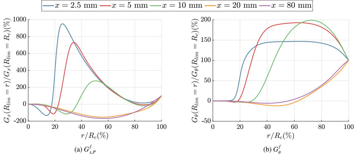
Figure 15: Effect of integration limit on the calculated flow rates  $G_{x,p}^f$  (left) and  $G_\theta^f$  (right) at five axial positions. The integral terms are computed by stopping the integration at various distances  $r$ , and then normalizing by the integral taken over the entire cross-section.  $p_{ref} = 101\,325.3$  Pa.
