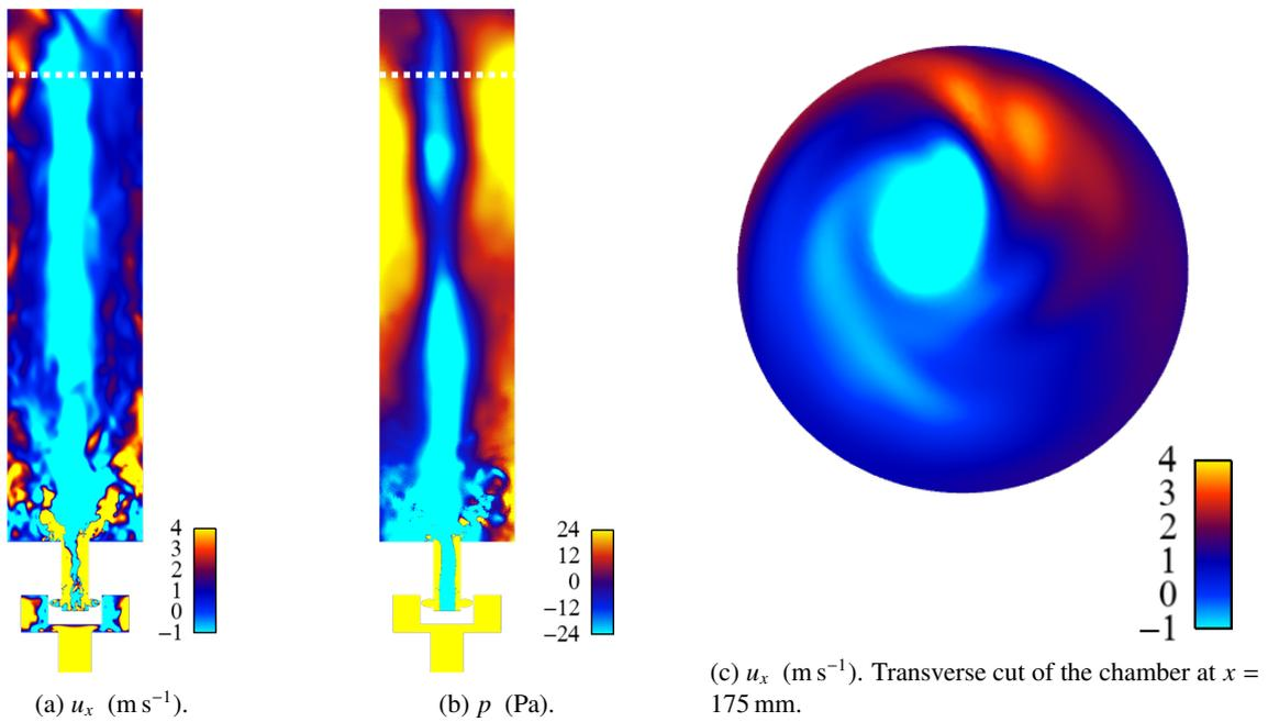
Figure 8: Axial cut showing the local instantaneous values of the axial velocity (a) and of the relative pressure,  $p - p_{atm}$  (b) in the chamber. The white dotted line in the chamber corresponds to  $x = 175$  mm, where a transversal cut showing the axial velocity near the outlet is taken and shown in (c).
