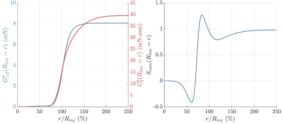
Figure 17: Choice of the integration limit  $R_{lim}$  for the computation of the conventional swirl number  $S_{conv}$  (Eq. (30)). Velocity profiles are taken at  $x = 2.5$  mm. On the left,  $G_{x,0}^0$  and  $G_{\theta}^0$  are plotted for different integration radii. On the right, the conventional swirl number  $S_{conv}$  is plotted in a similar manner.
