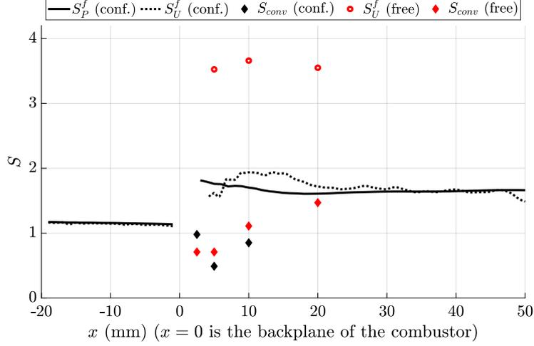
Figure 21: Comparison of different swirl numbers computed in the confined case (LES, black) and in the free jet (red, LDV).
