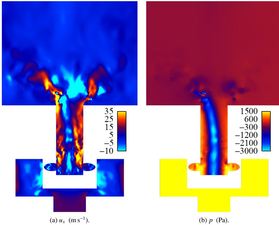
Figure 7: Axial cut showing instantaneous values of the axial velocity and of the pressure in the injector. Concerning the pressure, the atmospheric pressure  $p_{atm} = 101\,325$  Pa has been subtracted, and it is saturated at  $p_{atm} + 1500$  Pa as higher values are only reached upstream in the plenum.
