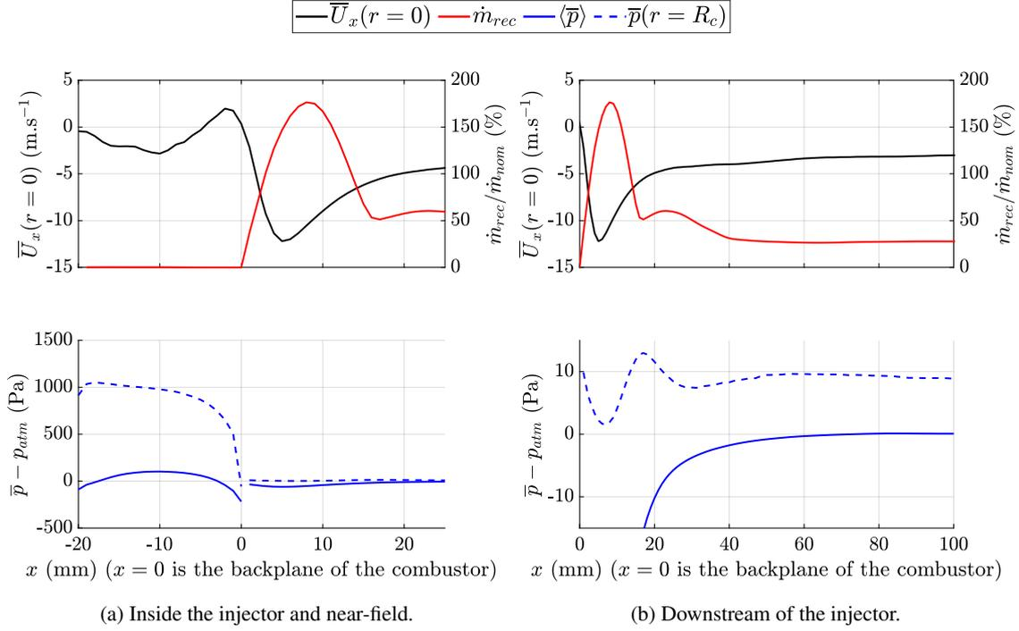
Figure 6: Top plot, left axis: evolution of the mean axial velocity  $\overline{U}_x$  on the centerline (black line); top plot, right axis: recirculating mass flow rate normalized by the nominal flow rate (red line); bottom plot: axial evolution of the section-averaged pressure  $\langle \bar{p} \rangle - p_{atm}$  (blue line) and of the pressure at the wall  $\bar{p}(r = R_c) - p_{atm}$  (blue dashed line).
