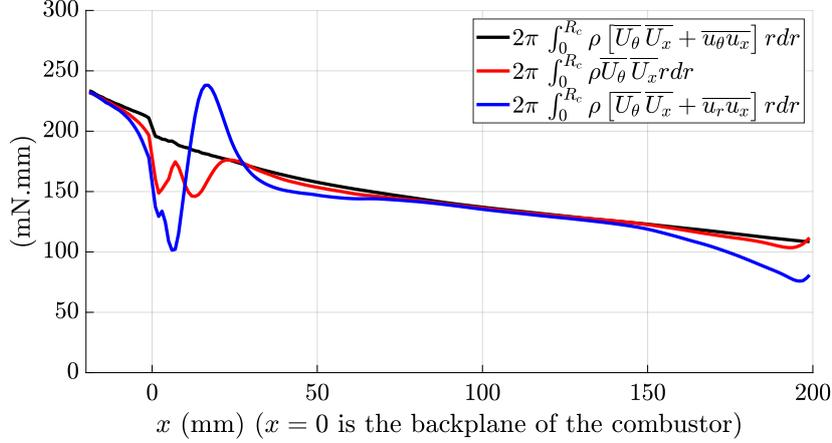
Figure 14: Assessment of the replacement of  $\overline{u_\theta u_x}$  by  $\overline{u_r u_x}$  in the computation of  $G_\theta^f$ .
