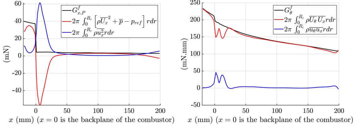
Figure 13: The different components of the flow rate of axial momentum (left) and axial component of the flow rate of angular momentum (right).  $p_{ref} = 101\,325.3$  Pa in the chamber ( $x > 0$ ) and  $p_{ref} = 101\,405$  Pa inside the injector ( $x < 0$ ).
