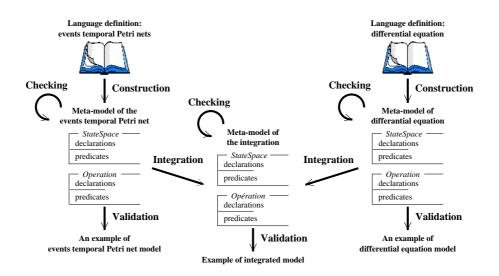
Fig. 2. Stages for meta-modeling a method
