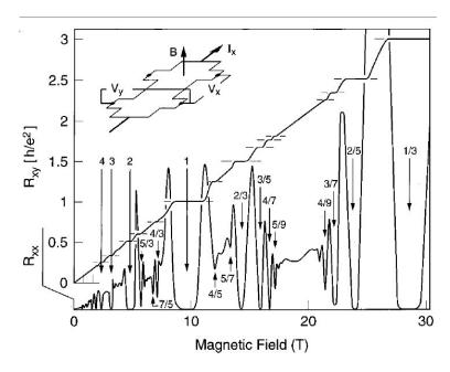
FIGURE 1. The fractional quantum Hall effect [51]. Sketch of the experimental sample in top-left corner. Plots of the longitudinal  $R_{xx} = V_x/I_x$  and transverse (Hall)  $R_{xy} = V_y/I_x$  resistances as a function of the magnetic field.
