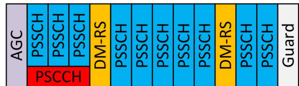
FIGURE 6. Long slot. For low speed, 2 DM-RS are enough to cover the whole slot. The front-loaded DM-RS symbol is shifted because no performance loss is expected in the interpolation and the edge extrapolation.
