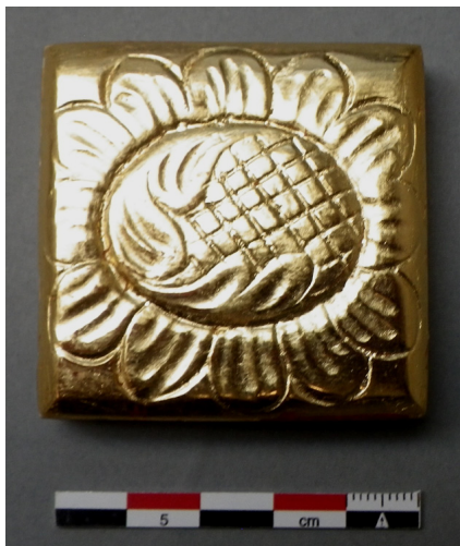
Figure 8. Specimen with the primer marked with \text{TiO}_2 and gilded half with traditional gold (left) and half with Au-Cu-In leaf (right). © C2RMF
