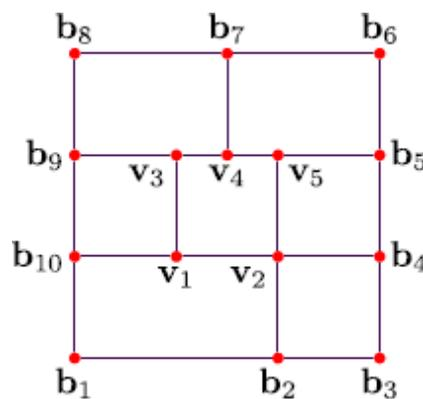
Fig. 1. An example of T-mesh.
