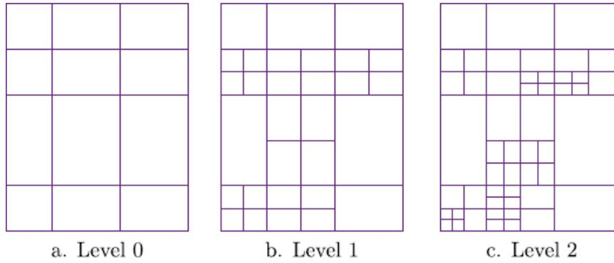
**Fig. 2.** A hierarchical T-mesh.
