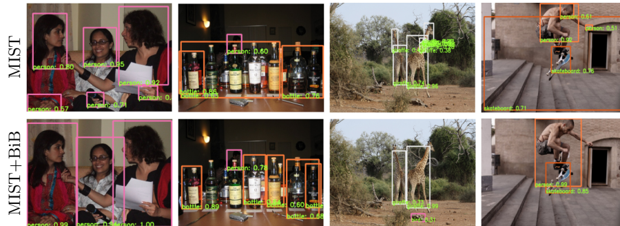
Fig. 5: Examples of predictions on the VOC07 and COCO test sets, by MIST [55] (first row) and BiB after the first cycle (second row). Fine-tuning MIST with images selected by BiB significantly remedies its limitations.
