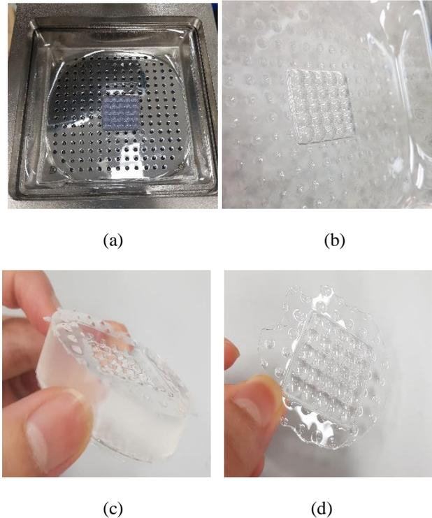
Fig. 2 Intermediate and final products from lens-making processes (a) the first lens prototype coated using vacuum forming machine (b) a lens prototype separated from the first prototype after vacuum forming (c) PDMS negative mould (d) a fabricated epoxy lens array after separation from the PDMS mould
