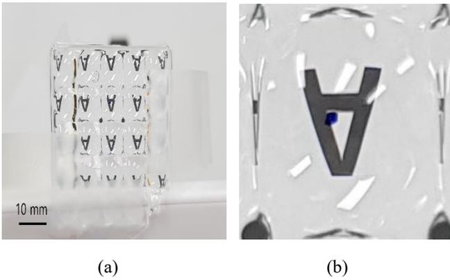
Fig. 3 Images of the letter ‘A’ formed by a fabricated lens array: (a) an image produced by the lens array with the tapes on the side for fixing the lens on the supporting structure. (b) a magnified view of the image produced by one of the lenses in the array with a marking dot on the surface
