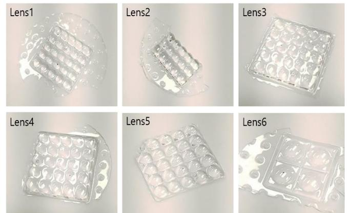
Fig. 5 Final epoxy lens arrays obtained from the first lens prototypes: Lens1 and Lens2 used prototype a with 0.6 mm and 1.0 mm thick plastic sheets, respectively; Lens3 and Lens4 used prototype b with 0.6 mm and 1.0 mm thick plastic sheets, respectively; Lens5 and Lens6 used prototypes c and d, respectively, with 1.0 mm thick plastic sheet.
