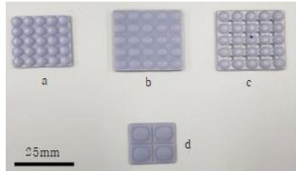
Fig. 4 Lens prototypes made by 3D printer: (a)  $r = 2.69$  mm ( $h = 1.7$  mm,  $d = 5.0$  mm), (b)  $r = 3.63$  mm ( $h = 1.0$  mm,  $d = 5.0$  mm), (c)  $r = 3.63$  mm ( $h = 1.0$  mm,  $d = 5.0$  mm), and (d)  $r = 6.63$  mm ( $h = 1.0$  mm,  $d = 10.0$  mm), where  $r$ ,  $h$  and  $d$  are the radius of curvature, lens height, and lens diameter, respectively; prototype c has same lens profile as that of prototype b but has holes between the lenses.
