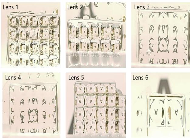
Fig. 6 Images of letter 'A' formed by the fabricated lens arrays
