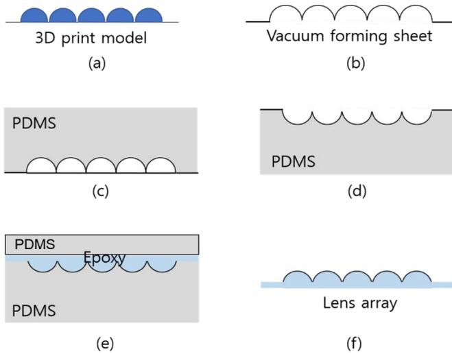
Fig. 1 Process flow involved in producing the lens array (a) making the first lens prototype using 3D printer (b) coating the prototype by vacuum forming (c) forming a negative PDMS mould (d) separating the PDMS mould from the lens prototype (e) pouring thermal epoxy into the PDMS mould (f) separating epoxy lens from the PDMS mould
