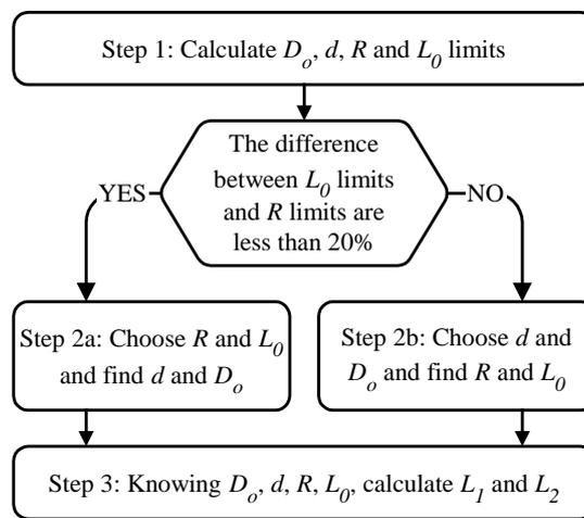
Fig. 4 Automatic determination of the starting point
