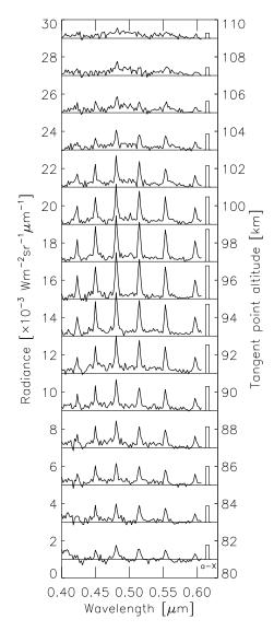
**Figure 4.** Spectra from all local times and all latitudes averaged over 2 km intervals for the tangent altitude from 80 km to 110 km. On the right, the corresponding a(0)-X(0) band intensities are shown on a linear scale. The line-of-sight c(0)-X(v'') and a(0)-X(0) intensities in the 94 km-96 km interval are 183.0 kR and 30.8 MR, respectively.
