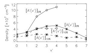
**Figure A1.** Number densities of the A(v'=0-7) and A'(v'=1-4) vibronic states of  $O_2$  in the  $CO_2/O_2/Ar$  flowing afterglow experiments by *Steadman and Thrush* [1994]. Densities with no  $CO_2$  added (solid lines). Densities with  $CO_2$  added at about 10% total pressure (dashed lines), i.e.,  $\sim 2.8 \times 10^{16}$  cm<sup>-3</sup>, which is the total number density at 88 km in Venus' atmosphere.
