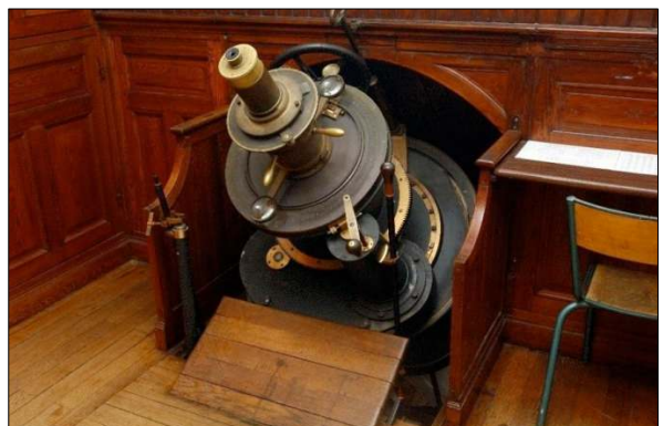
Figure 19: The focal environment of the Lyons coudé. Compare with Figure 9 (© Jean-Marie Refflé, DRAC Rhône-Alpes, 2004).
