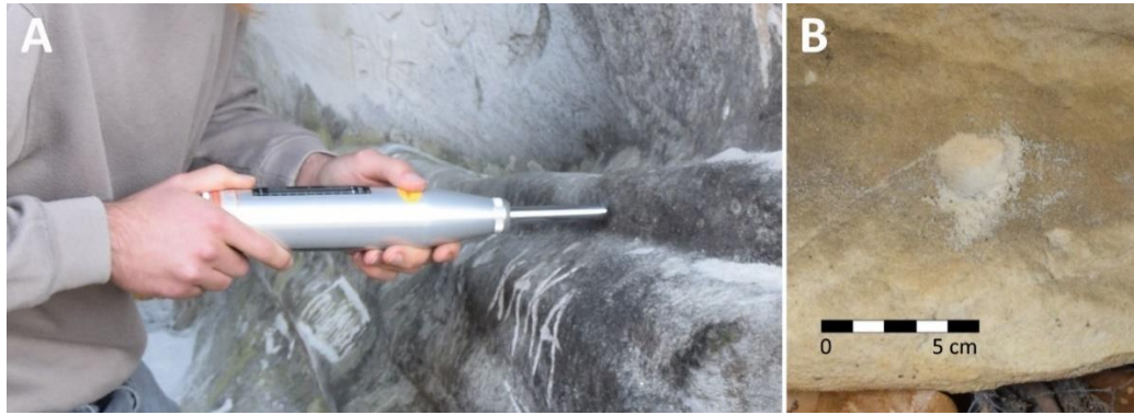
Figure 5: Measuring the hardness of sandstone. A: Schmidt Hammer during use on a boulder in a recent quarry. B: example of a cup mark impact left by a measurement on friable sandstone. [colour; 1 column]
