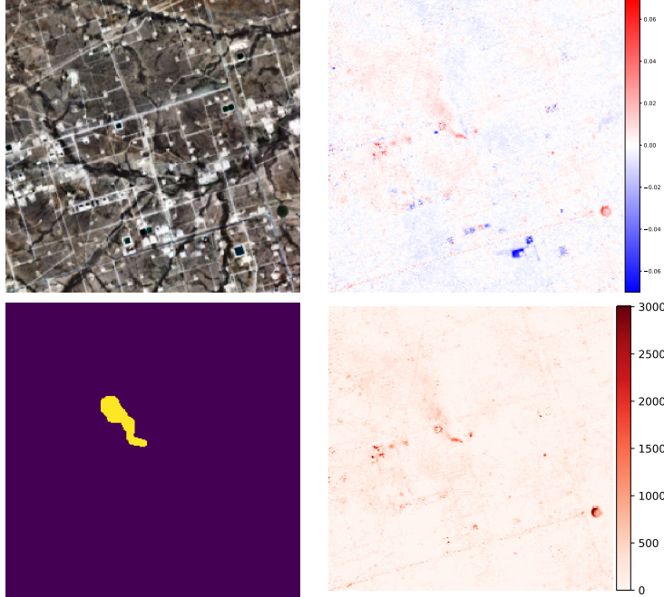
Figure 12: Visualization of each step of the detection and quantification pipeline. From left to right, top to bottom: the Landsat-8 image of the location (only the RGB channels are shown), the log band ratio corresponding to the image, the predicted background model, the residual showing the plume, the mask corresponding to the detected plume and the associated quantification in ppb.
