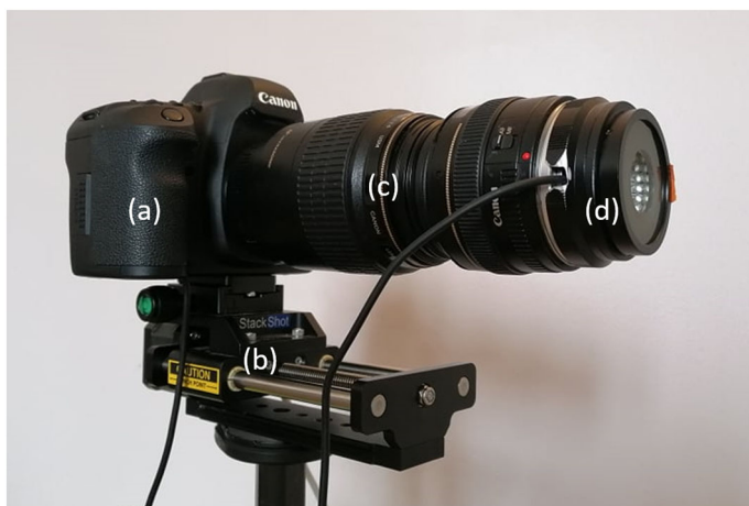
FIGURE 1 Acquisition device: (a) Canon EOS 5D II camera; (b) motorized rail; (c) optical system using a 100 mm lens and an inverted 50 mm lens; (d) light ring with diffuse filter
