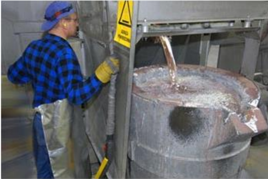
Fig. 1. Providing the molten alloys for the casting operation.
