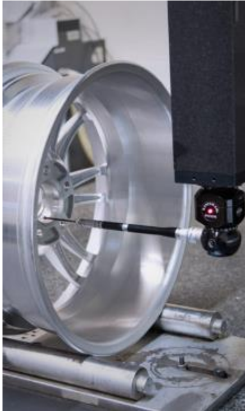
Fig. 4. Quality control of produced alloy wheels using the CMM.
