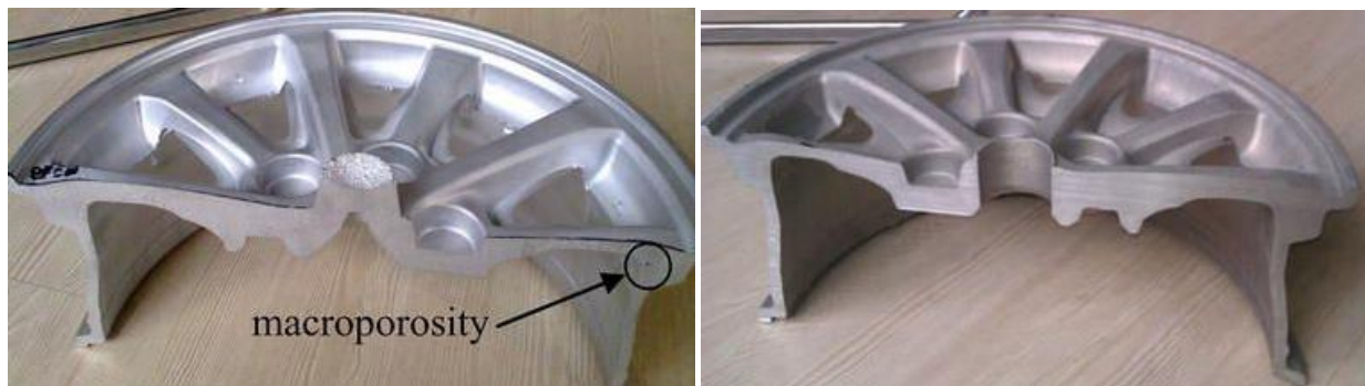
Fig. 13. Effect of the cooling and insulation process in removing the macroporosity defects in the junctions of produced alloy wheels [33].
