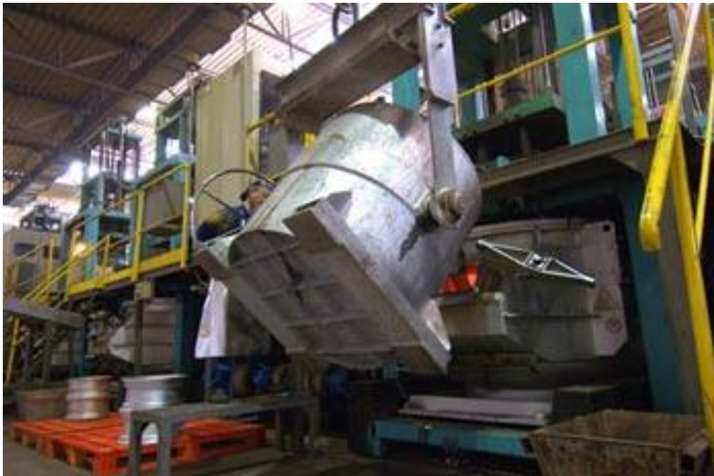
Fig. 2. Casting operation of wheel alloys.
