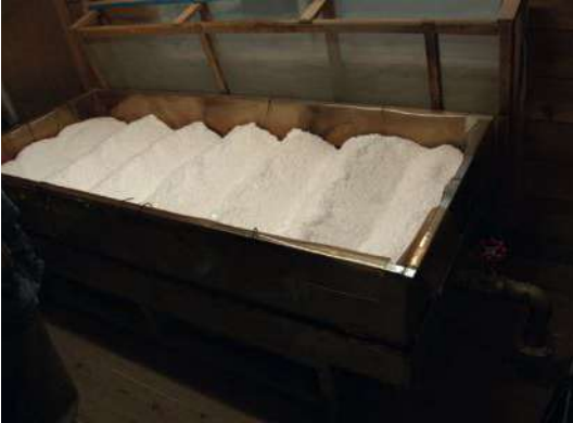
PHOTO 27 Salt formed into ridges in the drying pan to promote drying.
