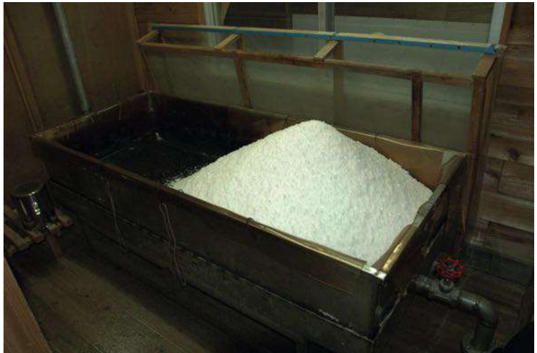
PHOTO 14 Geothermal drying pan.
