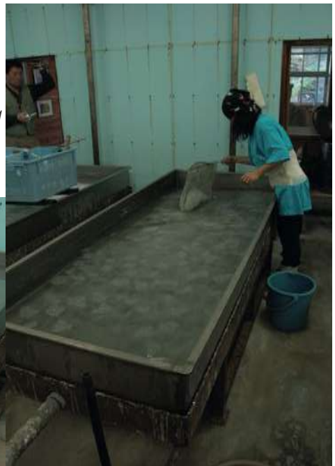
PHOTO 20 Removing calcium sulfate floating in a pan.
