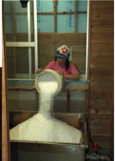
PHOTO 26 Dehydrated salt being transferred to the drying pan.
