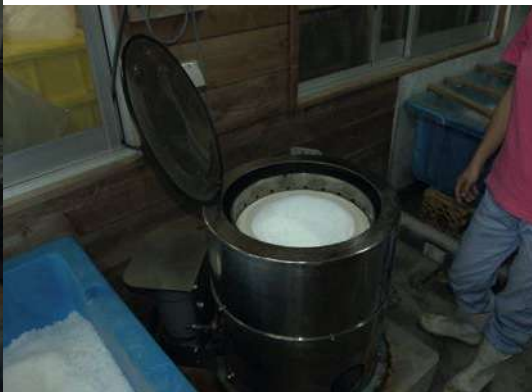
PHOTO 25 The dehydration bag is placed into the centrifugal dehydrator.
