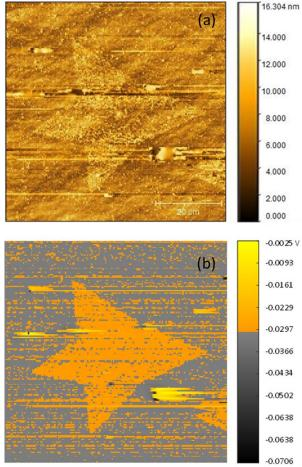
Fig 2. (a) Topography image obtained by atomic force microscopy with a Wollaston probe. A flat plane was subtracted from the raw image. (b) Raw thermal signal ( $\Delta V$ ) obtained during the same scan.
