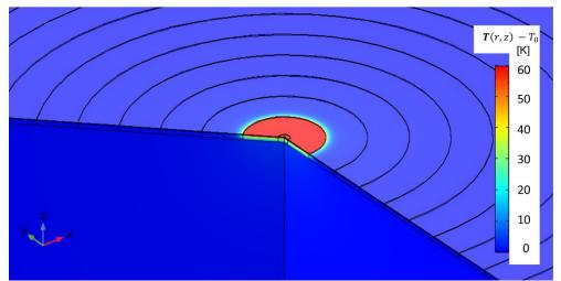
Suppl. Fig. 7. Temperature distribution on the equivalent (395 nm SiO<sub>2</sub> film on Si substrate) sample surface.
