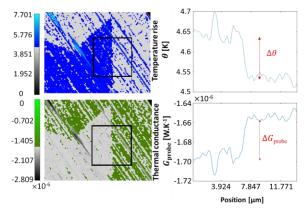
Figure 3. (Top) Probe temperature rise with respect to an arbitrary reference between the supported  $MoS_2$  and the silicaover-silicon wafer. (Down) Probe thermal conductance deduced from the temperature measurements (arbitrary reference). Left panels show rotated images with respect to Fig. 2, and right ones vertical averages in the square for each (horizontal) position.
