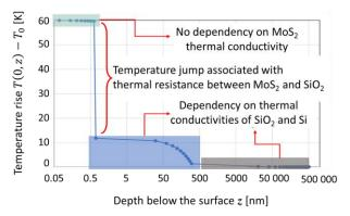
Figure 4. Temperature profile in logarithmic scale as a function of depth below the heat source (FEM simulation). The upper region overlaid in green corresponds to the  $MoS_2$  monolayer, the lower blue region corresponds to SiO<sub>2</sub>, and, finally, the gray region corresponds to the contribution of the Si substrate.
