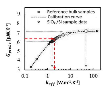
Suppl. Fig. 6. Variation of the probe thermal conductance (reference far from contact) as a function of the effective thermal conductivity.
