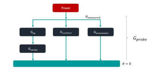
Suppl. Fig. 4. Suppl. Fig. 3. Thermal circuit associated with heat dissipation in the probe.
