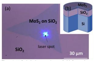
Figure 1. (a) Optical microscopy image of a  $MoS_2$  monolayer with a triangular shape. The light dot corresponds to a laser spot irradiating the surface. (b) Cross-section schematic of the analyzed system.
