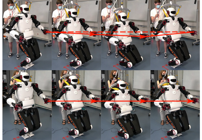
Fig. 1. Comparison of squat trajectory performance between hand-tuned control parameters (top) and parameters learned using our method (bottom), on the Talos robot.
