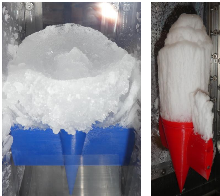
Figure 17 : sample of ice produced in realistic condition left: glaze ice, U_{air} = 80\text{m/s} , T = -5.3^\circ\text{C} , LWC = 0.54 , MVD = 20\mu\text{m} right: rime ice, U_{air} = 80\text{m/s} , T = -30^\circ\text{C} , LWC = 0.54 , MVD = 20\mu\text{m}
