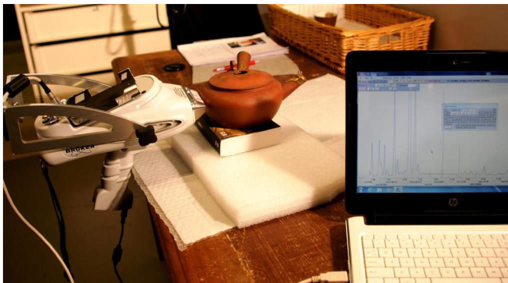
Figure 2. View of the measurement set-up. The XRF spectrum was evaluated after recording on the laptop screen.
