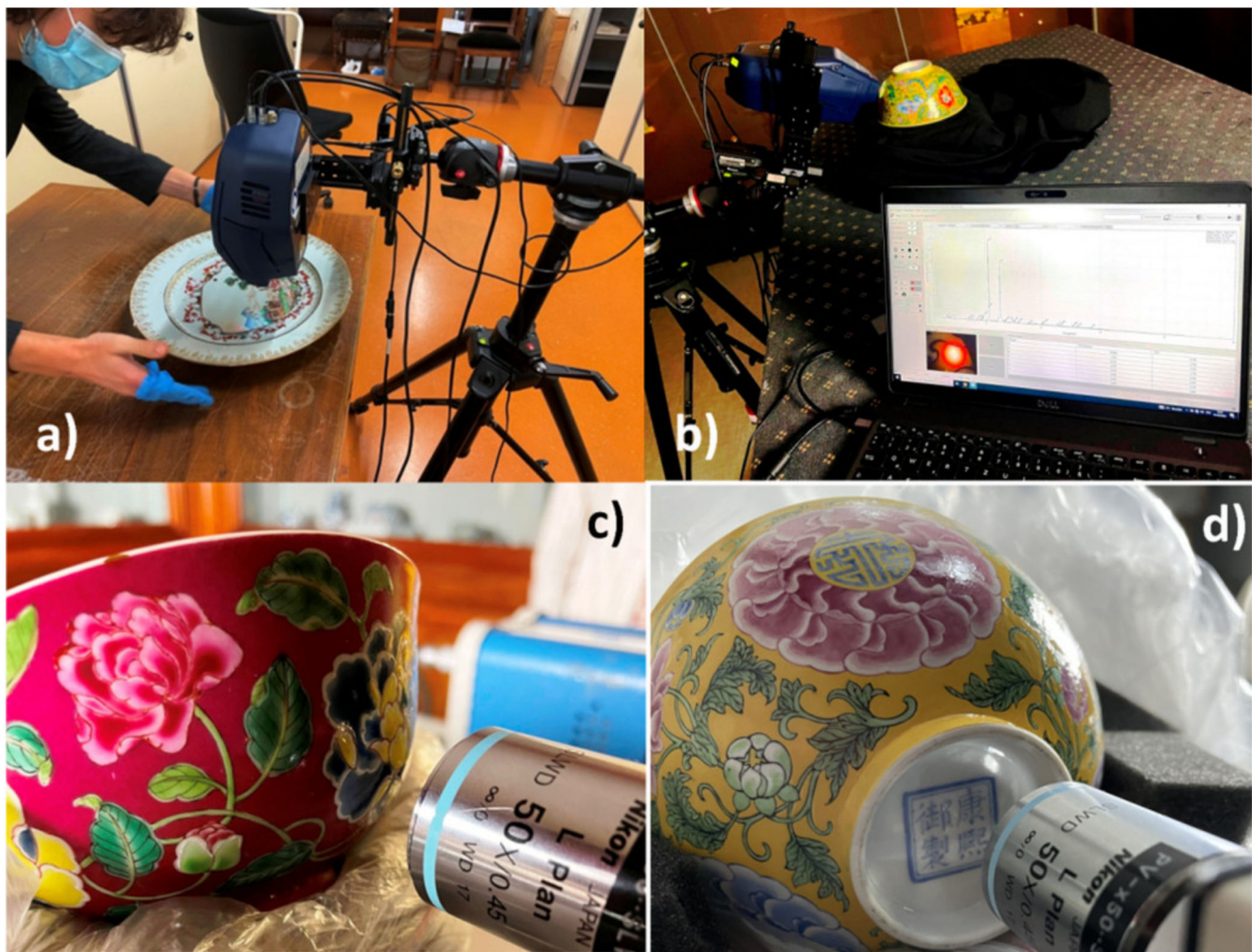
Figure 1. View of the XRF analysis set-up, the measurement can be made from top (a) or side (b), the orientation of the instrument being variable and the XY displacement motorized and computer-controlled; (c,d) views of the Raman analysis, from the decoration or the mark by using a 50× microscope objective. See references [10–13,50] for more details about the mobile Raman set-up.
