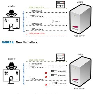
FIGURE 7. SlowDrop attack (based on [56]).
