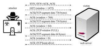
FIGURE 5. Slow read attack (based on [52]).
