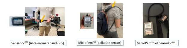
Figure 5. Data collection sensors. In the left side, Sensedoc<sup>TM</sup> sensor (Accelerometer and GPS) which should be worn in a belt around the waist. In the middle, MicroPem<sup>TM</sup> (pollution sensor) which should be worn in a bag or purse with the pipe as close to the airway as possible. In the right side, the MicroPem<sup>TM</sup> and the Sensedoc<sup>TM</sup>.
