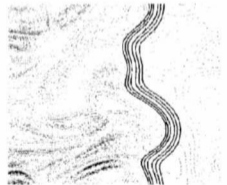
Flame artificially thickened by a factor \mathcal{F}
