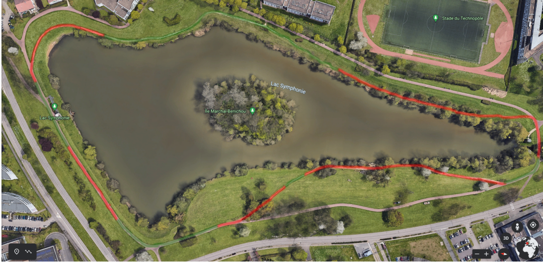
Figure 22: Red: areas where ICP keyframe building was inconsistent or failed, without semantic knowledge. Green: Areas where semantic-aware ICP was not necessary for successful keyframe reconstruction.
