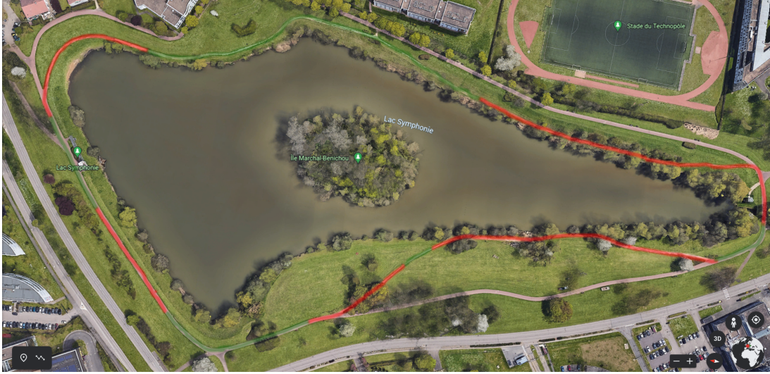
Figure 22: Red: areas where ICP keyframe building was inconsistent or failed, without semantic knowledge. Green: Areas where semantic-aware ICP was not necessary for successful keyframe reconstruction.
