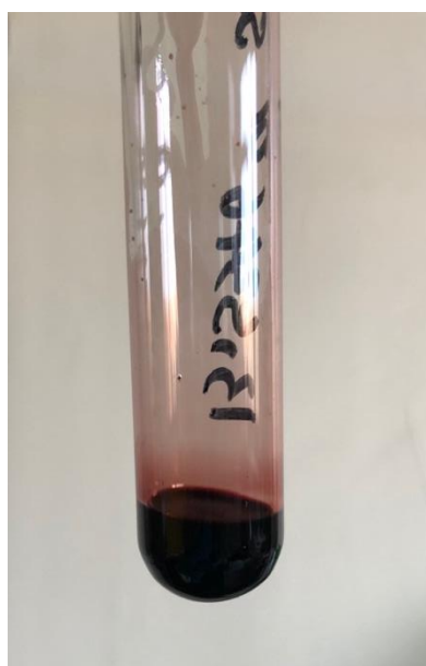
Figure S10. Photograph of CuNPs prepared in the presence of 5 equiv. of \text{PPh}_3 at 65\text{ }^\circ\text{C} in \text{CHCl}_3 after centrifuging.
