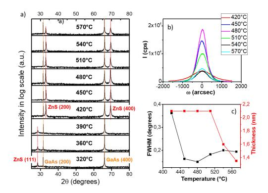
**Figure 2.** X-ray diffraction analysis of ZnS layers grown at various temperatures, from 320°C to  $570^{\circ}$ C : a)  $\theta$ -2 $\theta$  scans, b)  $\omega$ -2 $\theta$  rocking curves, and c) full width at half-maximum and layer thickness plots, as a function of the growth temperature
