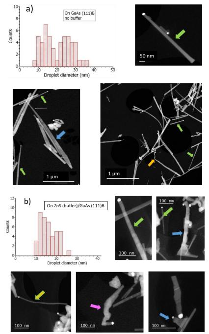
**Figure 8.** STEM/HAADF image and droplet diameter statistics of ZnS NWs grown on: a) GaAs (111)B, and b) ZnS (buffer)/GaAs (111)B.
