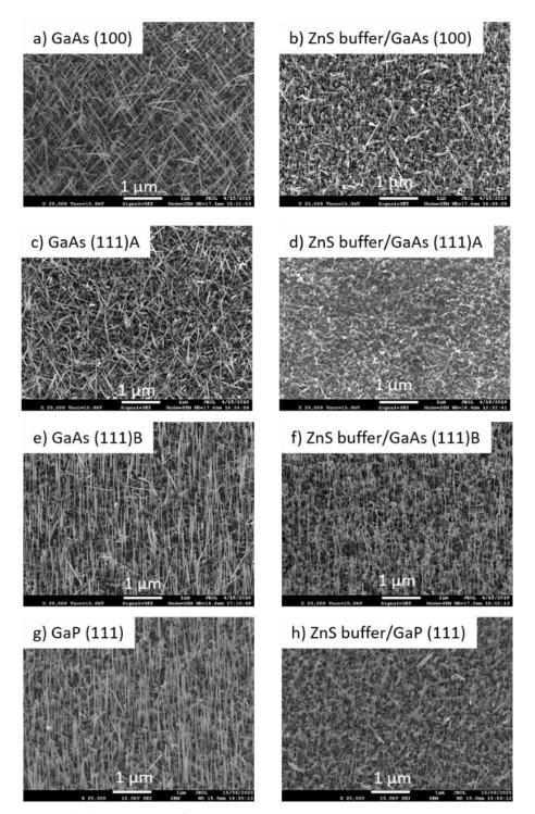
**Figure 7.** 45° tilted SEM images of ZnS NWs grown on GaAs (100), GaAs (111)A, GaAs (111)B, GaP (111), and ZnS buffers.
