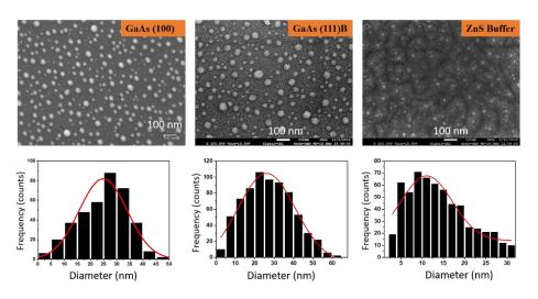
**Figure 3.** SEM images and statistics of gold droplets deposited and dewetted on GaAs (100), GaAs (111)B, and ZnS/GaAs (111)B substrates.
