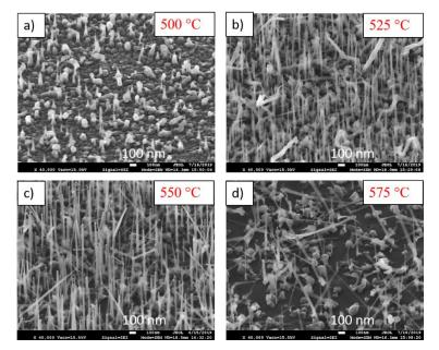
**Figure 5.** 45°-tilted SEM image of samples prepared on GaAs (111)B sustaining RvI/II = 2 at different temperatures : a) 500 °C, b) 525 °C, c) 550 °C and d) 575 °C.
