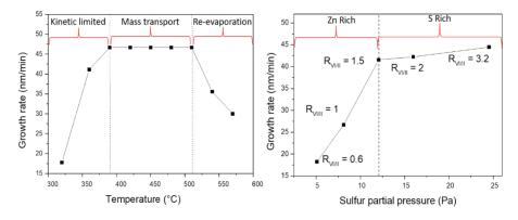
**Figure 1.** Growth rate of ZnS thin films as a function of : a) substrate temperature, and b) DTBS partial pressure.
