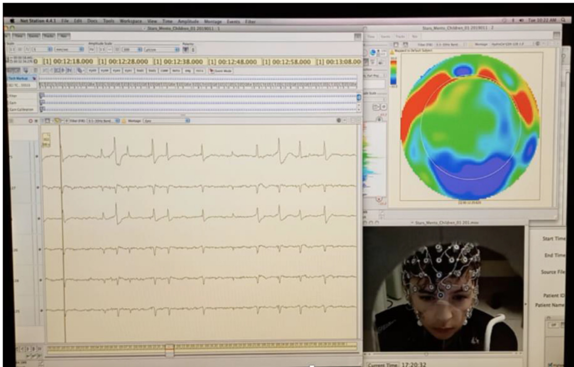
Fig. 2. Snapshot of a video-EEG recording collected in a 5-year-old child while executing a cognitive task. The left panel shows the online EEG recording with a detailed view of the electrodes around the eyes. The top-right panel displays the online topographical spline map, while the bottom-right shows the EEG-synchronized eye behaviour (EGI© system). The EEG recording is taken from a dataset originally published by Timeo, Mento, Fronza, and Farroni, 2018.
