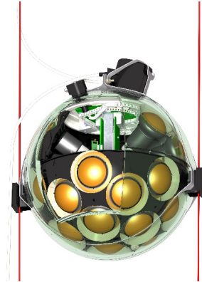
Figure 4. Rendition of an optical module mounted with bollards attached to the supporting ropes of a detection unit. For illustration purposes, several parts are cut out. The breakout-box which connects to the backbone cable of the detection unit (see section 3.4) is attached to the top of the module.
