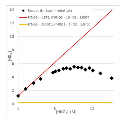
Figure 2: Effect of the integration of the contribution of HNO<sub>2</sub> to the model of the system studied with Phreeqc with different equilibrium constants and comparison with experimental values from Ruas et al.
