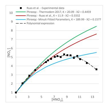
Figure 1: Comparison between Phreeqc calculated values with the database Thermoddem 2017 (green curve), with K°<sub>HNO3-Ruas</sub> (red curve), with MINUIT fitted parameters (blue curve), with empirical polynomial function (dotted curve) and with the experimental data from Ruas et al. (black squares) of HNO<sub>3</sub> dissociation
