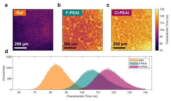
Fig. 4 Time-resolved photoluminescence imaging analysis. a-c Map of decay time obtained on full-stacks (glass/ITO/PTAA/perovskite/BCP/PCBM) for the high fluence (1.5 × 10<sup>12</sup> ph.cm<sup>-2</sup>) acquisition. The homogeneity of the A-cations devices is comparable to the neat reference cell. **d** Histogram of the maps, showing the passivation effect of the layers.
