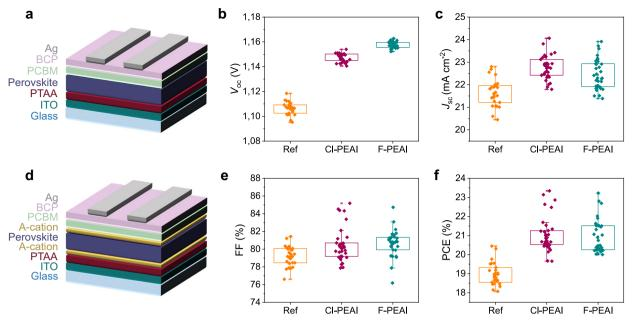
**Fig. 1 Electrical characterisation of the samples. a** Schematic of the reference samples **d** Schematic of the A-cation p-i-n devices with dual interfacial modification. Photovoltaic characteristics of reference (orange), CI-PEAI (purple) and F-PEAI (teal blue) devices. **b** Open circuit voltage ( $V_{oc}$ ). **c** Short circuit current ( $J_{sc}$ ). **e** Fill Factor (FF). **f** Power conversion Efficiency (PCE).
