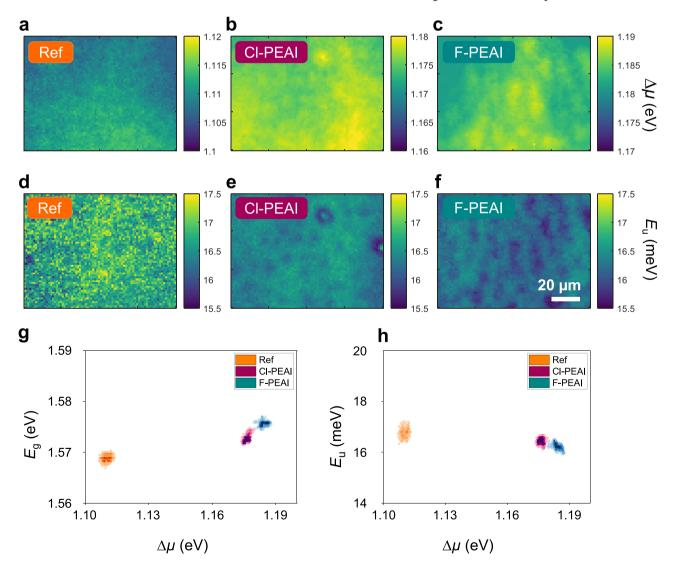
Fig. 3 Continuous wave photoluminescence imaging analysis. Hyperspectral measurements on the stack glass/ITO/PTAA/perovskite/BCP/PCBM. quasi-Fermi level splitting ( $\Delta\mu$ ) maps for **a** reference sample, **b** CI-PEAI and **c** F-PEAI samples. Urbach Energy maps for **d** reference sample, **e** CI-PEAI and **f** F-PEAI samples. **g** Correlation between energy gap and QFLS. **h** correlation between Urbach Energy and QFLS. The scalebar applies to all images.
