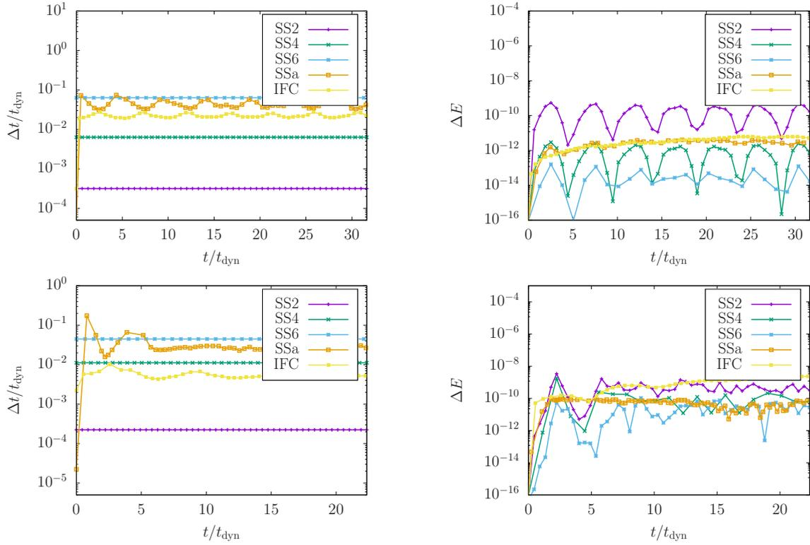
Figure 2: Comparison for the 1D SN equation between the time-step and the error on the energy conservation for the IFC method and the Split-Step solvers for both the cases  $g = 10$  (upper plots) and  $g = 500$  (lower plots).
