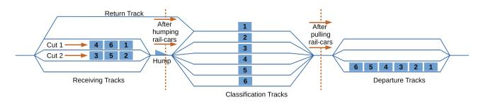
FIGURE 10 Three main steps of the sorting-by-block algorithm
