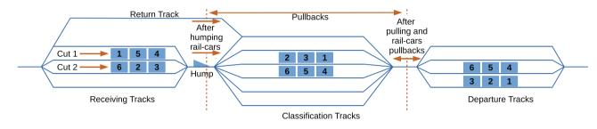
FIGURE 11 Three main steps of the sorting-by-train algorithm
