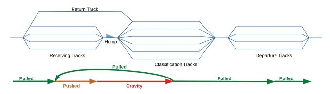
FIGURE 6 Schematic representation of the actions/forces moving cars in the different part of the layout
