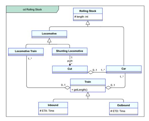
FIGURE 2 UML class diagram: rolling stock
