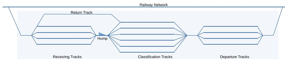
FIGURE 1 Schematic representation of a typical yard
