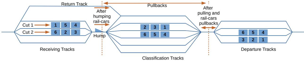
FIGURE 11 Three main steps of the sorting-by-train algorithm
