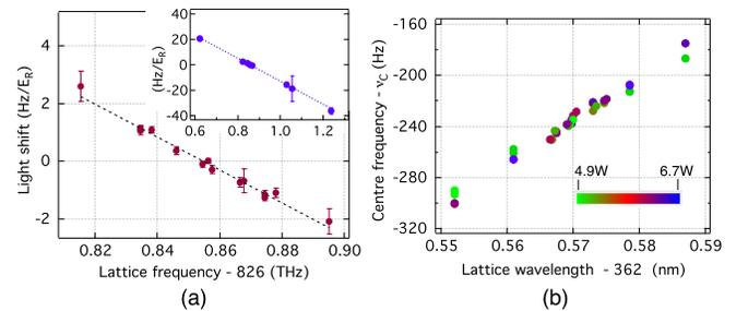
FIG. 4 (color online). (a) Differential light shift versus lattice frequency for the  $^{199}\text{Hg}$  clock transition. The inset shows measurements made over a larger frequency range. The Stark-shift free frequency (wavelength) is  $826.8546 \pm 0.0024$  THz ( $362.5697 \pm 0.0011$  nm) and the slope is  $-57\ \text{mHz } E_R^{-1} \text{ GHz}^{-1}$ . (b) Clock transition frequency versus lattice wavelength with changes of lattice power. ( $1\text{W}$  implies  $3.5E_R$  for the trap depth.)
