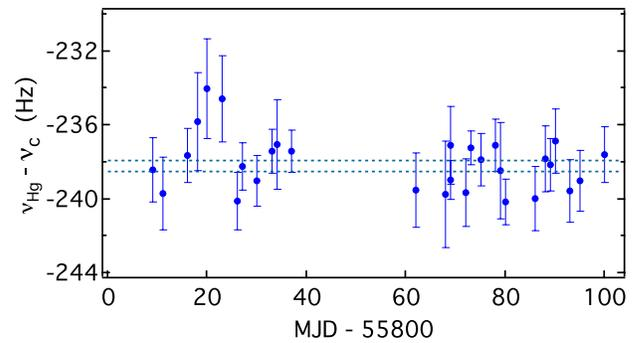
FIG. 6 (color online). Clock transition frequency measured over a three month period with respect to the SYRTE primary frequency standard for  $\lambda_m = 362.5697$  nm. The weighted mean is  $\nu_c - 238.2 \pm 0.3$  Hz.  $\nu_c = 1\,128\,575\,290\,808\,400$  Hz.
