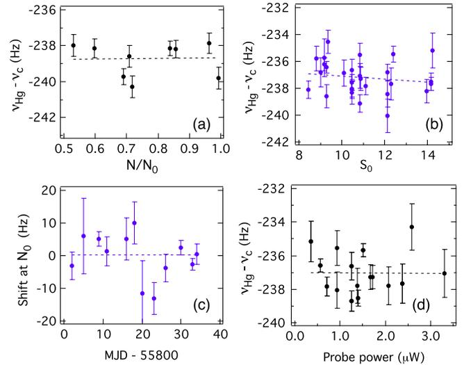
FIG. 5 (color online). Line-center frequency versus (a) relative atom number, where  $N_0 = 2.5 \times 10^3$  and (b) MOT cooling light intensity,  $s_0$ . (c) Frequency shift at  $N_0$  versus measurement day. (d) Line-center frequency versus probe power.
