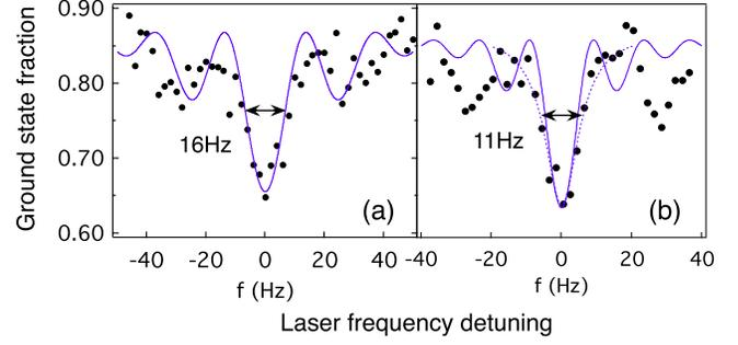
FIG. 3 (color online). Ground state fraction versus probe laser detuning frequency for (a) 50 and (b) 80 ms Rabi pulses.  $\Omega_p T_p = 1.45\pi$  and  $1.36\pi$  rad for the curve fits (solid lines), respectively.  $B = 0$  and  $\lambda_L \approx \lambda_m$  for (a) and (b).
