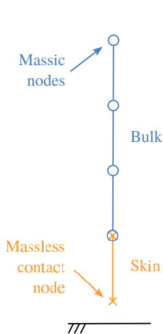
Figure 1: Redistributed mass on a discrete bar
