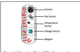
Figure 1– Schematic of Digital Pill with a range of potential sensors and other devices.
