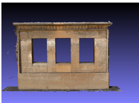
Figure 13. Resulting dense point cloud with archives photographs combined to contemporary photographs.
