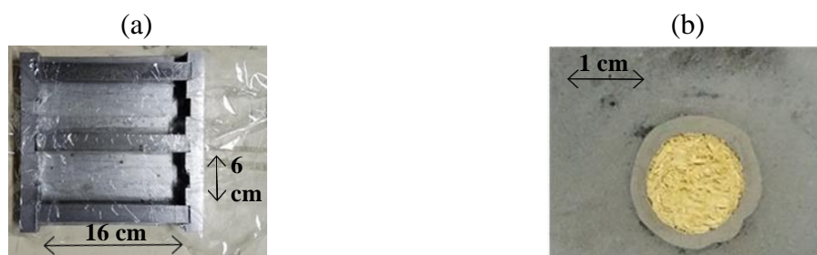
Figure 4. (a) Mold and plastic film to pour the cement paste and (b) pellet cast in cement paste after cement setting.
