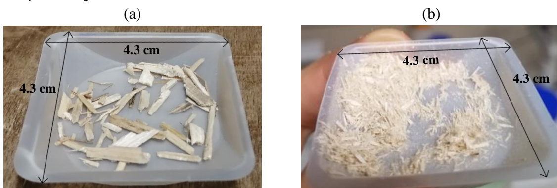
Figure 3. Photos of 0.1g (a) raw hemp shives and (b) hemp after grinding.
