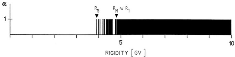
Fig. 5.4 Function \alpha(R) for the station Jungfraujoch for vertical direction of incidence and corresponding cutoff rigidity values: R_S (Störmer cutoff), R_M (main cutoff), and R_1 (first-discontinuity rigidity)
